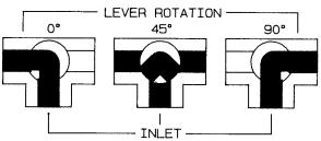
NOTE: Open port pressure must exceed Closed port pressure.
